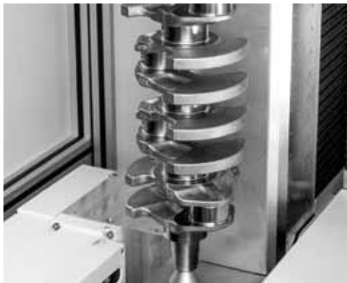
HOMMEL-ETAMIC opticline CA618-AE; designed specifically for measuring crank shafts
