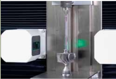
Measuring a turbo-charger
