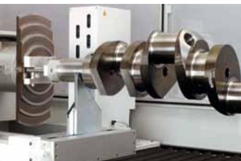
HOMMEL-ETAMIC opticline WMS, solution with a horizontal design and a crank shaft application
