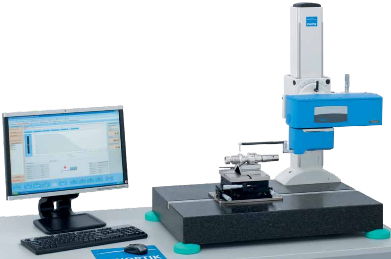
HOMMEL-ETAMIC T8000 C120-400 digiscan with optional measuring table MT1 XYO and vee-block
