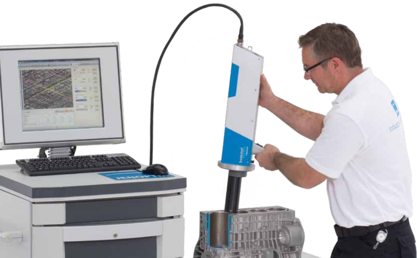
HOMMEL-ETAMIC toposcan OR150 with mobile workstation
