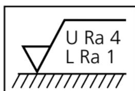
Material removing machining; upper and lower limit value for Ra demanded; Ra = min. 1  $\mu\text{m}$  and max. 4  $\mu\text{m}$
