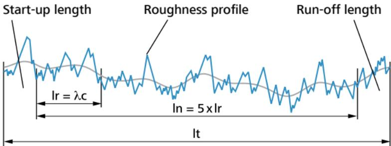
The traverse length ( $l_t$ ) is the total length of the probe movement during the scanning process. It must be greater than the evaluation length  $l_n$  in order to be able to form the roughness profile with the profile filter. With the exception of  $R_t$ ,  $R_{mr}(c)$  and  $R_{Pc}$ , the roughness parameters are defined within an evaluation length  $l_n$ , which is determined using an average of five sampling lengths  $l_r$ .
