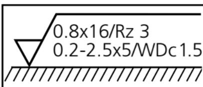
Material removing machining; Rz: the evaluation length is 12.5 mm and  $\lambda_c = 0.8$  mm, Rz = max. 3  $\mu\text{m}$ ; WDc: in the period range of 0.2 to 2.5 mm, WDc = max. 1.5  $\mu\text{m}$  applies
