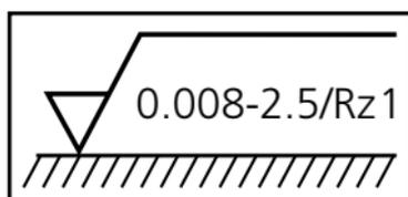
Material removing machining; transmission characteristic does not comply with standard case (cf. table) Rz = max. 1  $\mu\text{m}$ ; filter selection  $\lambda_s = 0.008$  mm and  $\lambda_c = 2.5$  mm
