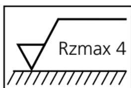
Material removing machining; Rz = max. 4  $\mu\text{m}$ ; the maximum value rule applies
