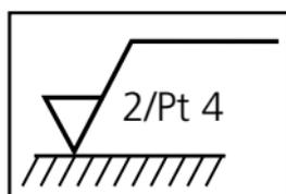
Material removing machining; P-profile, traverse length = 2 mm; Pt = max. 4  $\mu\text{m}$
