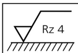
Material removing machining;
