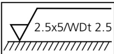
Material removing machining; in the period range up to 2.5 mm, WDt = max. 2.5  $\mu\text{m}$  applies
