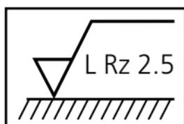
Material removing machining; lower limit value for Rz demanded;
